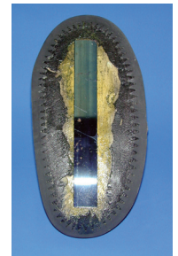
Spring steel sole stiffeners.
